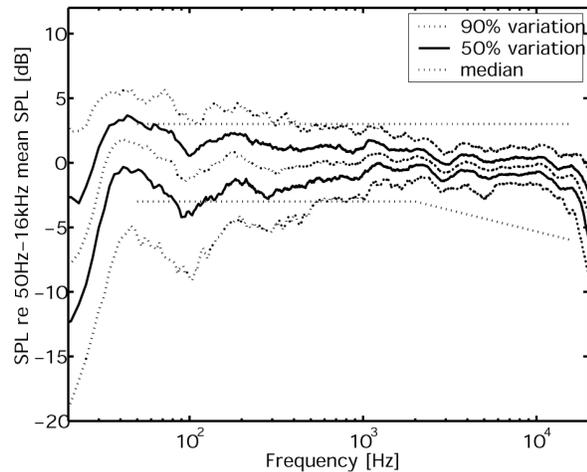
Fig. 7. Third octave smoothed sound pressure level measured at the listening position ( $N = 250$ ) for speakers aimed at the listening position. 50Hz-16kHz mean level normalized to 0dB. Also shown are German Surround Sound Forum proposed limits (dotted line).
