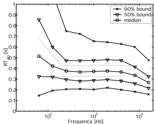
Fig 3. 90% and 50% bound limits and the median for reverberation time  $RT_{60}$  in octave bands ( $N = 372$ ). German Surround Sound Forum limit shown (dotted line) centered at the median of mean  $RT_{60}$  levels.
