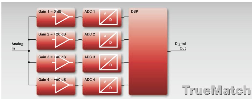
Fig.: Principle of the TrueMatch converter
